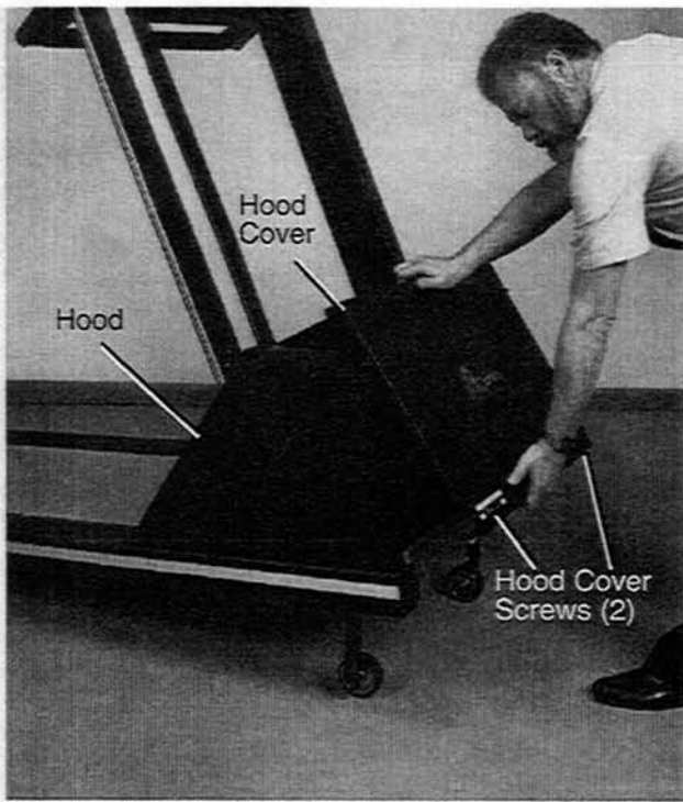
Figure 3-1. Removing Treadmill Hood Cover
